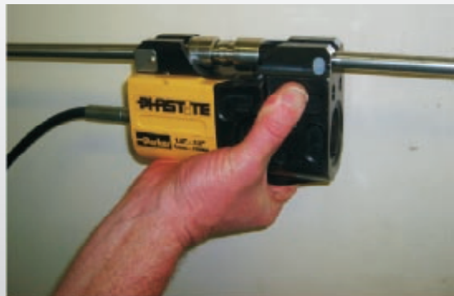
Figure 2. Phastite tooling allows assembly direct against panels and bulkheads.
